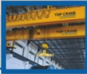
DOUBLE GIRDER EOT CRANE
