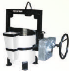
Gear Ladle Cap. 250 kg to 5 Ton
