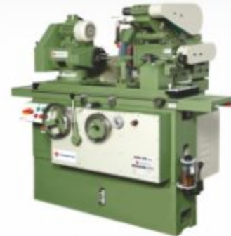
Cylindrical Grinding Machine 150 x 300 mm
