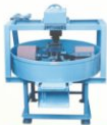
Muller Machine Cap. 50kg., 1 Ton
